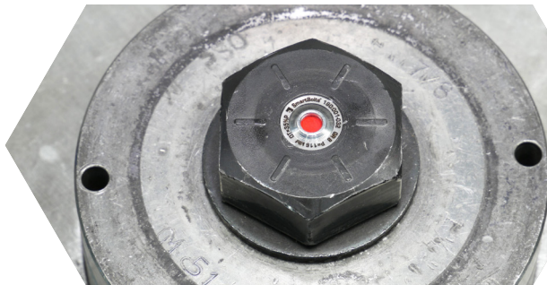
SmartBolt at zero tension
